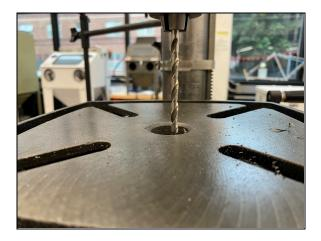
5.2.4. Position one of the marked hole locations on the spool beneath the tip of the drill. Clamp the spool to the table in this position. Clamp the center of the spool as shown in the image below so that the clamping force is supported by the center cylinder of the spool and not the free edges.
